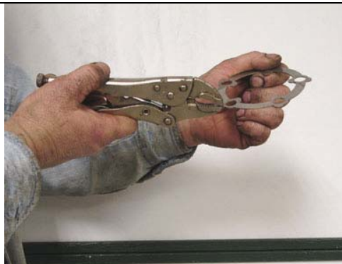
Step 15: using a vise grip, bend the tabs on the lock ring up slightly. Trust me, this will help you later.
