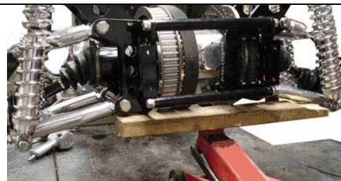
Step 22: Lift the unit up using a rolling jack, or a stack of wood. Slide it forward and line up the three holes on the adjuster plates.
