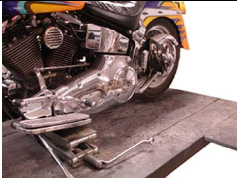
Step 1: Secure bike and jack rear wheel off the ground. Be sure to leave access to both ends of the shocks.
